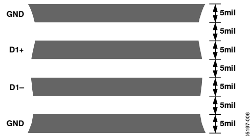
Figure 18. Arrangements of Signal Tracks
